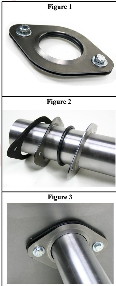
This floor mount is designed to mount a steering column to the floor or firewall and can be installed on either side of the body.
