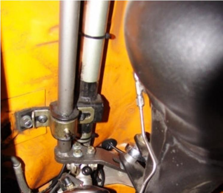
1. Bolt the sway bar arms to the bar using three 5/16" x 1 1/4" bolts, Nylok nuts and flat washers per side.
