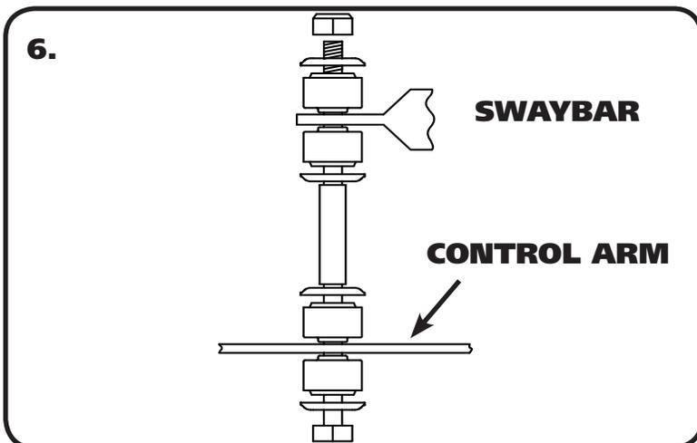
6. Install the End Links. Use Diagram "6" for proper installation. Tighten the Hex Nut enough to slightly compress the Bushings.
