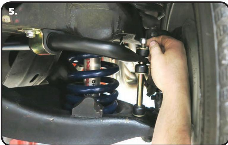
5. Install the End Links. Use the photo in Diagram "5" and Diagram "6" for proper installation. The Threads on the bolt should point up. Tighten the Hex Nut enough to slightly compress the Bushings.
