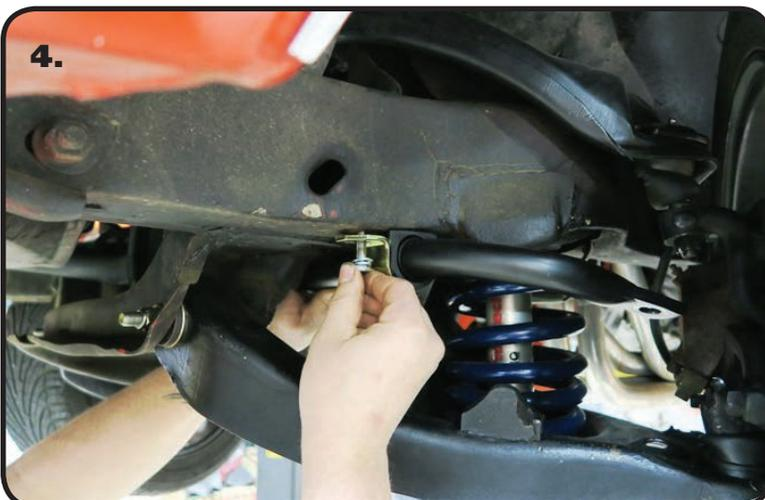
4. Slide the SwayBar into position on the Car. You may need to move the bushing assemblies on the swaybar to get the slots in the straps to align with the OEM threaded holes. Install a 5/16" Lockwasher and 5/16" Flatwasher on each 5/16" Bolt and thread them into the OEM Threaded holes. Do **NOT** Complete tighten the Hardware. It will be left partially loose until the End Links are installed.
