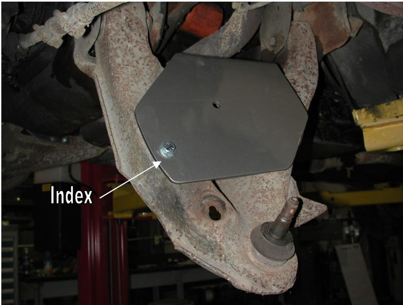
6. Set the air spring plate on the lower control arm. The plate will index off of the factory bump stop hole. Insert a  $3/8"$  x  $1\ 1/4"$  with Nylok and flat washers.
