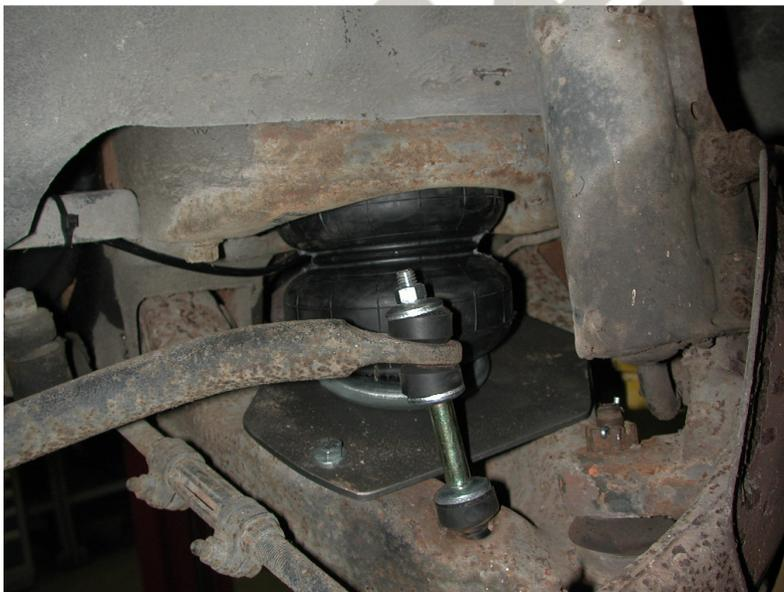
12. Place the air spring into the pocket with the stud protruding through the hole you drilled earlier. The air fitting should point towards the engine. It is held in place with a  $7/16"$  Nylok and flat washer.
