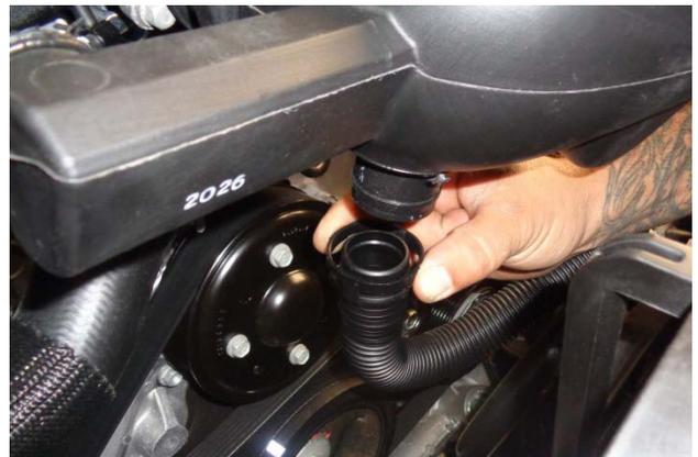
11. Disconnect the resonator hose from the bottom of the intake duct by squeezing the locking ring and pulling straight down.
