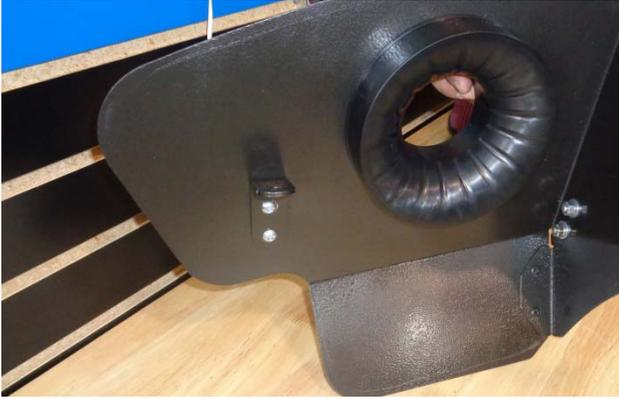
19. Attach bracket (8) to airbox using ¼-20 screws (10) (on the bracket side), and flat washers (3), lock washers (4) and nuts (5) (on the airbox side).
