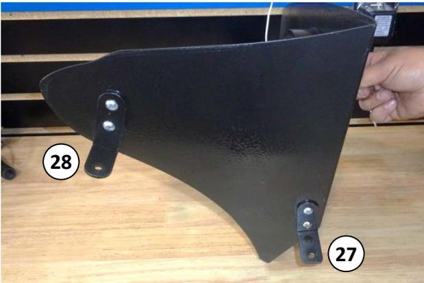
20. Attach brackets (28) and (27) to airbox using ¼-20 screws (10) (on the bracket side), and flat washers (3), lock washers (4) and nuts (5) (on the airbox side).
