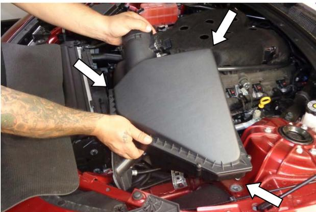
9. Grasp each corner of the airbox (at the arrows), one at a time, and firmly pull straight up to release each mount pin from its rubber grommet. After releasing all three pins, remove the airbox.
