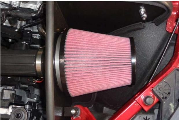
32. Place clamp (2) on air filter (1), install filter on filter adapter and tighten clamp.
