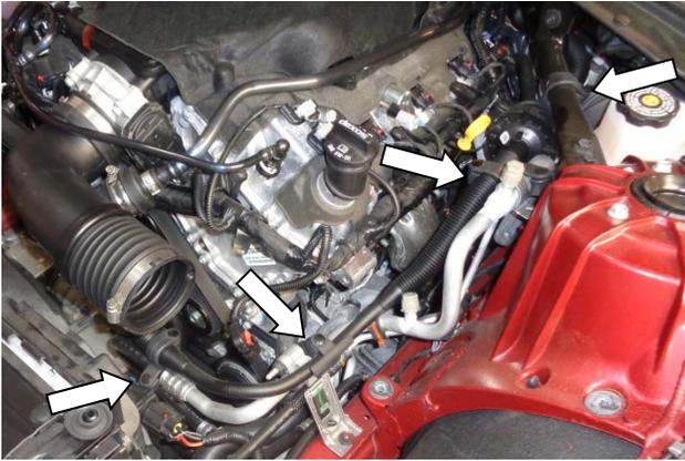
13. Disconnect the four clamps shown, and remove the resonator and hose from the vehicle. (The clamps may be left attached to the resonator and hose.)
