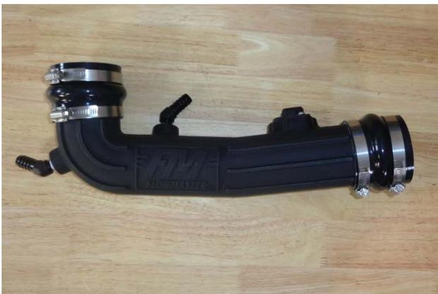
27. Install two hose clamps (20) on each coupler (13), and install couplers on each end of intake tube.
