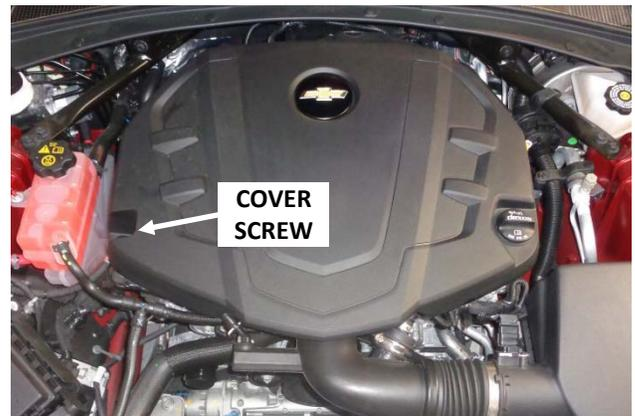
4. Remove engine cover screw and oil fill cap.
