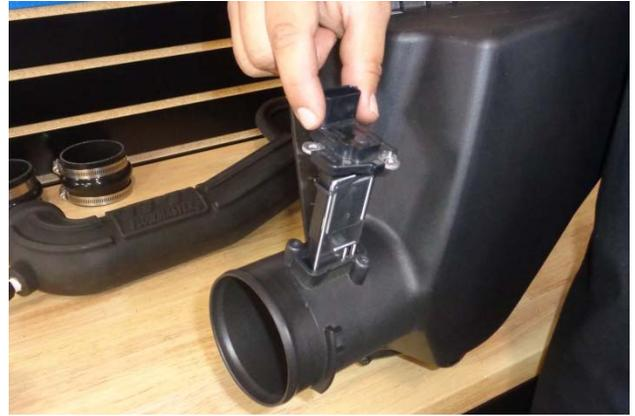
16. Remove the MAF sensor from the airbox, then remove the stock gasket from the sensor.
