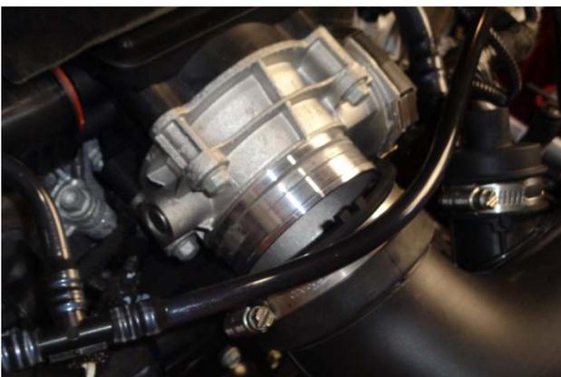
15. Loosen hose clamp securing the air intake duct to the throttle body. Disconnect the duct from the throttle body, and remove the duct from the vehicle.
