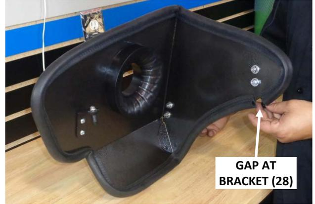
22. Attach gasket (26) to heat shield. Starting on one side of bracket (28), firmly press the gasket onto the edge, gradually working around the heat shield. When you reach the other side of the bracket, trim the gasket to fit using metal-cutting shears.
