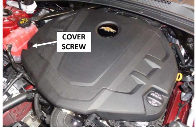
34. Reinstall oil fill cap and engine cover screw.
