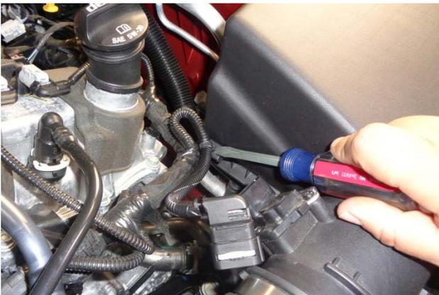
8. Release the clip that secures the MAF sensor lead to the airbox.
