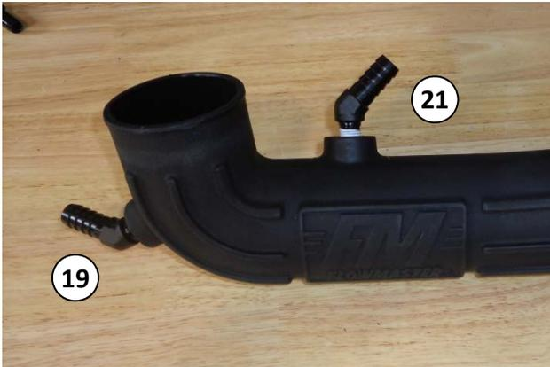
25. Apply 2 wraps of nylon thread tape to threads of 1/2" elbow (19) and 5/8" elbow (21), and install them into the intake tube (15) at the locations shown.
