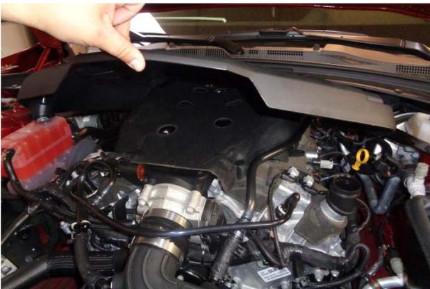
33. Remove oil fill cap and reinstall engine cover.
