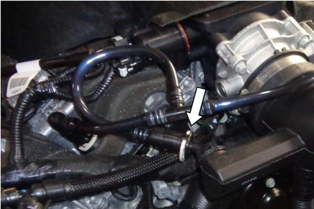
14. Disconnect the EVAP system hose from the intake duct.
