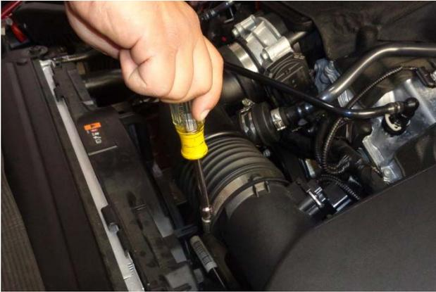
7. Loosen the hose clamp securing the air intake duct to the airbox, and disconnect the duct from the airbox.
