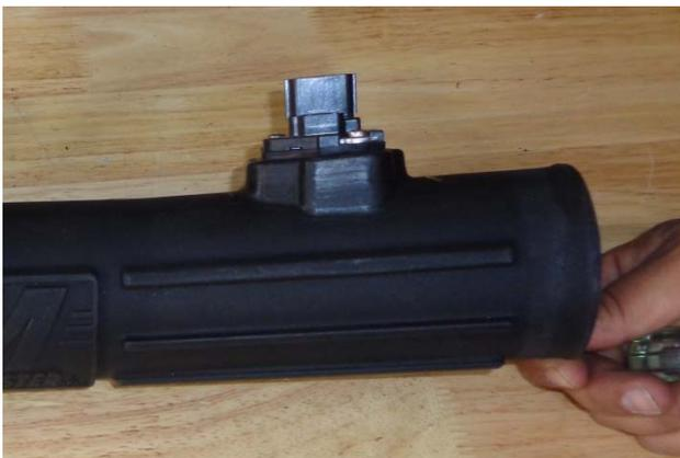
26. Install MAF sensor gasket (25) onto the sensor, ensuring correct orientation. Then install sensor in intake tube, using M4 screws (24).
