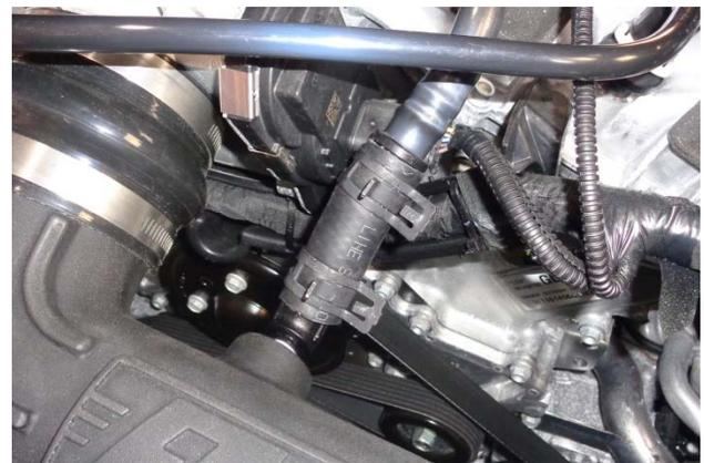
30. Install one end of 5/8" ID hose (23) on 5/8" elbow and secure with pinch clamp (22). Cut hose to fit to PCV hose fitting. Secure hose to PCV fitting with pinch clamp (22).
