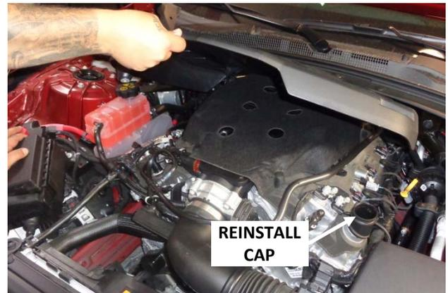
5. Remove engine cover, then reinstall oil fill cap.
