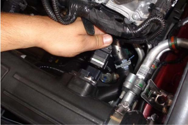
31. Install MAF sensor plug on sensor, and push locking tab toward the sensor. Check plug for security.
