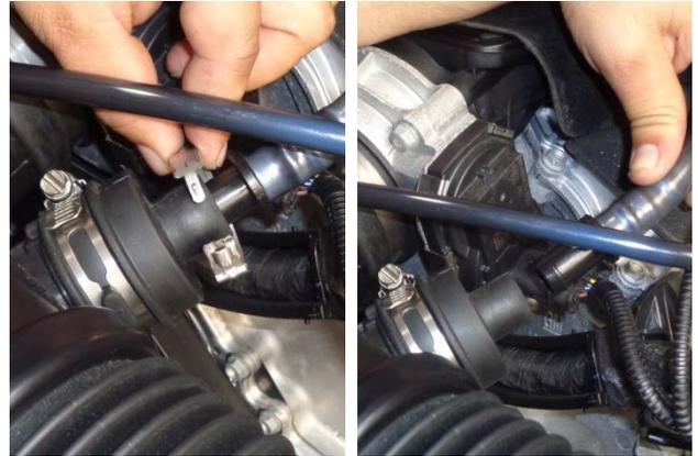
10. The PCV hose clamp is not reusable. Carefully cut and remove the clamp, then disconnect the hose from the intake duct.
