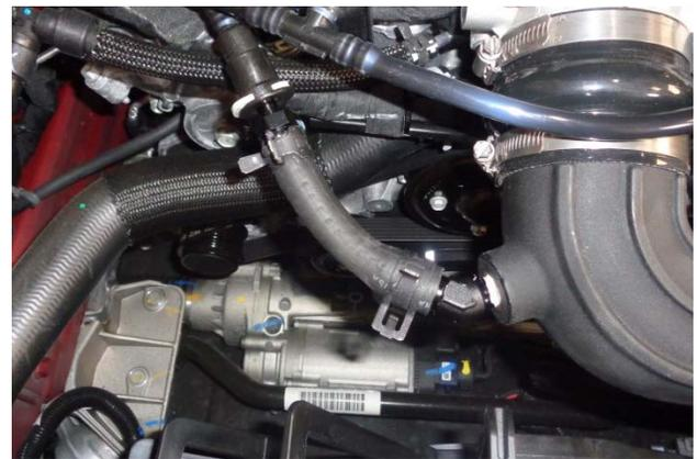
29. Install quick-disconnect fitting (17) in one end of 1/2" ID hose (18) and secure with pinch clamp (16). Cut hose to fit between EVAP hose connector and 1/2" elbow. Secure hose to elbow with pinch clamp (16), and connect QD fitting to EVAP hose connector.
