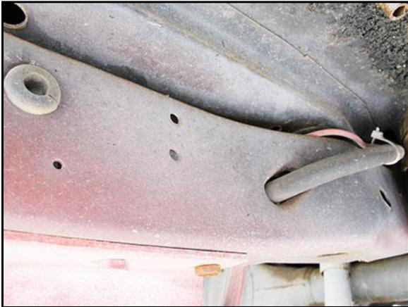
Figure 5 – Right side frame attachment holes
