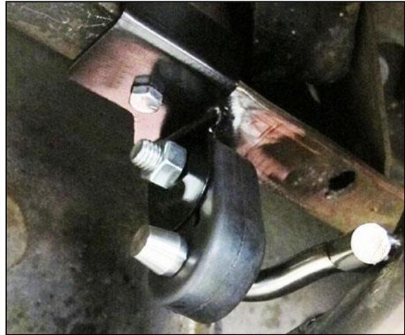
Figure 4 – Right tailpipe hanger bracket
