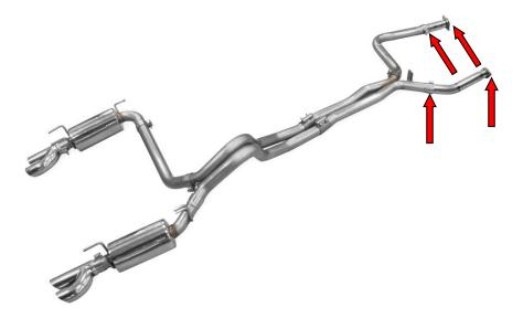
6. **For existing BlackHeart RACE ONLY Exhaust:** Loosen the (x4) band clamps securing the frontmost pipes to the BlackHeart Exhaust System and BlackHeart Mid-Length Headers. Remove the frontmost pipes.
