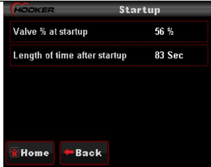
Press Valve % at startup bar and use the slider to set the valve position to 0 %
