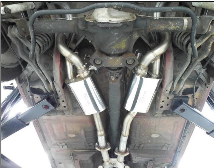
**Figure 3 – Mid mount install w/ tailpipes**
