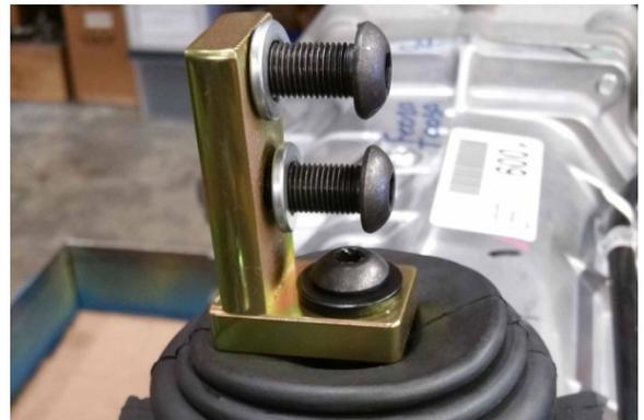
Attach the Chrome Hurst shift handle to the lower stub stick using the supplied hardware. This shifter locates the handle in nearly the same location as the stock shifter hole in the floor. There may be some modification required to the floor or tunnel area to accommodate the larger size of the Tremec transmission.
