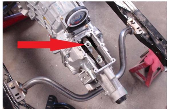
When you are sure your shifter is correctly positioned, apply a new bead of RTV sealer to the lip of the shifter cavity and mount the shifter by re-using the six, 5/16" bolts. Torque the bolts to 20 ft/lbs.
