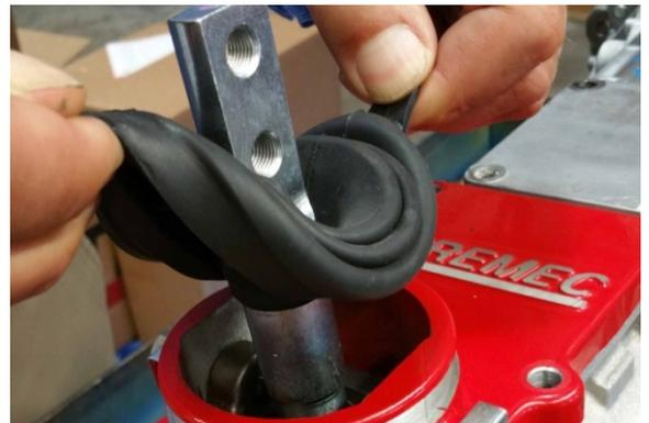
The shifter "body" will be in the forward position on the rear T56 shifter cavity. Make sure the pivot ball is positioned into the rear socket and that the white plastic bushing is still in place.
