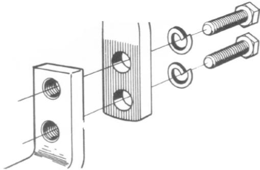
Stick bottom with tapped holes do not require stiffener plate.
