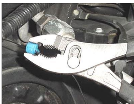
Figure 5 (Close T-Tap connector)
